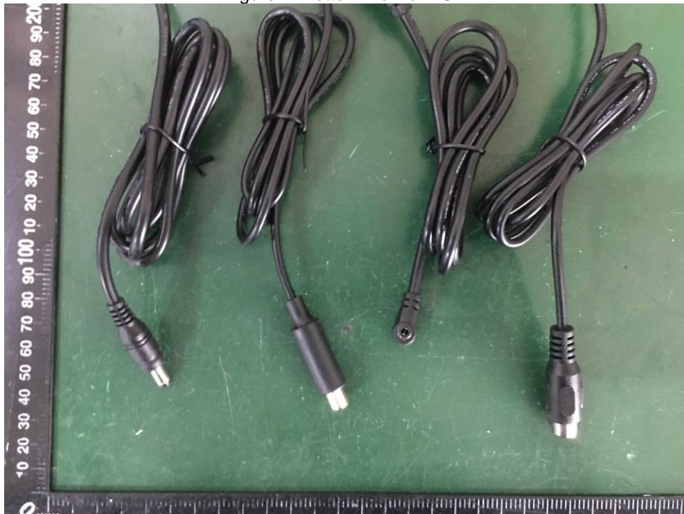
Figure 8. Output terminal for unit (Output \leq 42V )
