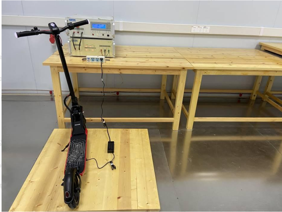
Photo of Surge Immunity Test
