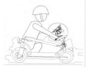
Fold the scooter so that the hooks hang onto the backsplash notches.
