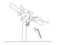
Adjust the handlebars and tighten the screws with a hexagon wrench to avoid loosening.
