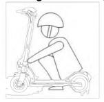
Hold the steering column and pull outward the folding hook of the column.
