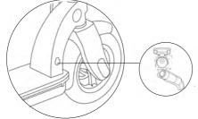
Find the charging port on the edge of the deck and plug in the charger
