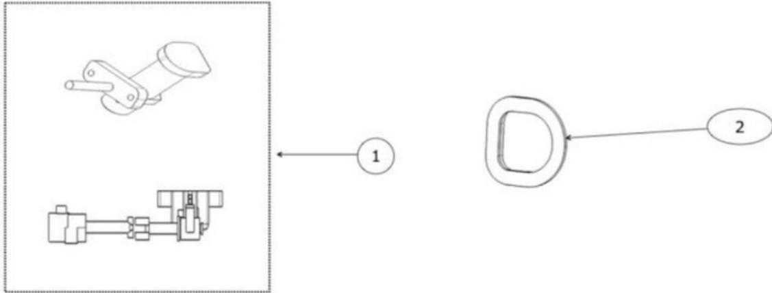
1 ● ENSEMBLE CONTACT ET FERMETURE SIÈGE (S02-46126-00)
